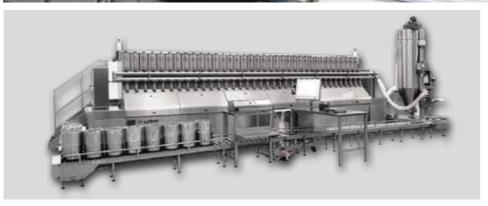
is a fully automatic weighing system for powder ingredients, granting constant quality and thorough control over food preparations.
